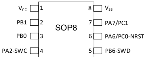
图 3-7 SOP8 Pinout1 PY32F002BL15Sx ( Top view )
